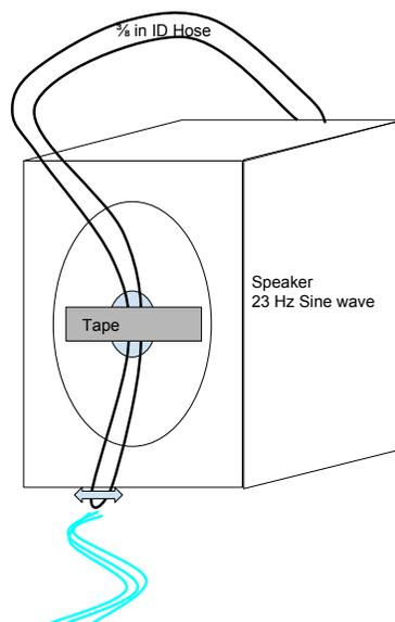
The Flow exiting tube was disrupted by the 23 Hz vibrations from the speaker causing the water to fall as a sine wave. This falling sine wave is very difficult to see with the naked eye, however, a camera filming at a similar frequency can cause the water wave to appear stopped, or move backwards or forwards. For this video, a 23 Hz sound wave was placed through the speaker while the camera filmed at 24 fps, making the sine wave appear to move backwards, towards the water source.
