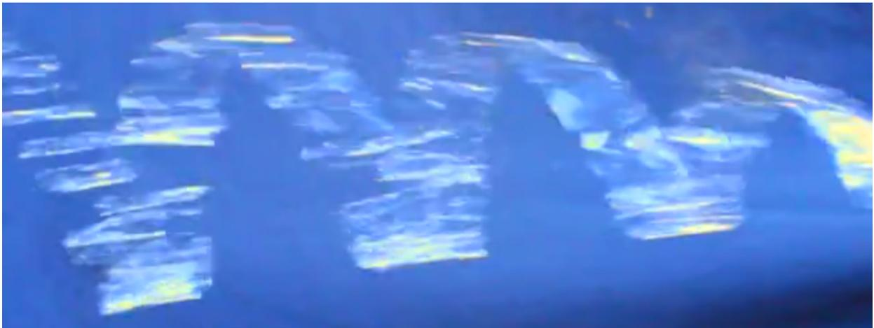
This is the first group project done by John Zeldes, Rachael Grosskrueger, and Brock Derby. The purpose of this video is to show a freeze frame of oscillatory fluid flow. It shows how a fluid falling in the form of a sine wave of different frequencies can appear to freeze in time by filming at similar frequencies to the fluid flow. This experiment was inspired by “Amazing Water and Sound Experiment #2” filmed by “Brusspup” and shows this phenomenon captured using higher camera shutter speeds.
